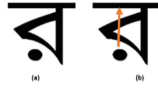
Fig. 6. (a) Dot as a part of text (b) scanning of upper region for context information.
