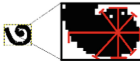
Fig. 9. Determination of stroke width along four directions. The red lines correspond to the continuity in pixels along a particular direction. (Color figure online)
