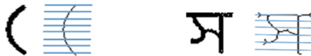
Fig. 8. Demonstration of row-wise scanning of a skeletonized bracket and non-bracket component. Here, for the bracket, no row encounters a significant number of data pixels. This is because a bracket is generally written in a single stroke as shown.
