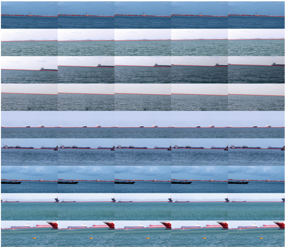
Fig. 6. The red line indicates the horizon detected by proposed method.
