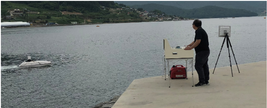
Fig. 3. The experiment of using directional antenna prediction control system at sea
