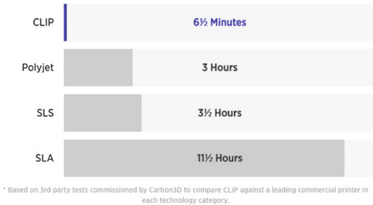
Fig. 40.1 Printing time for different printing technology
