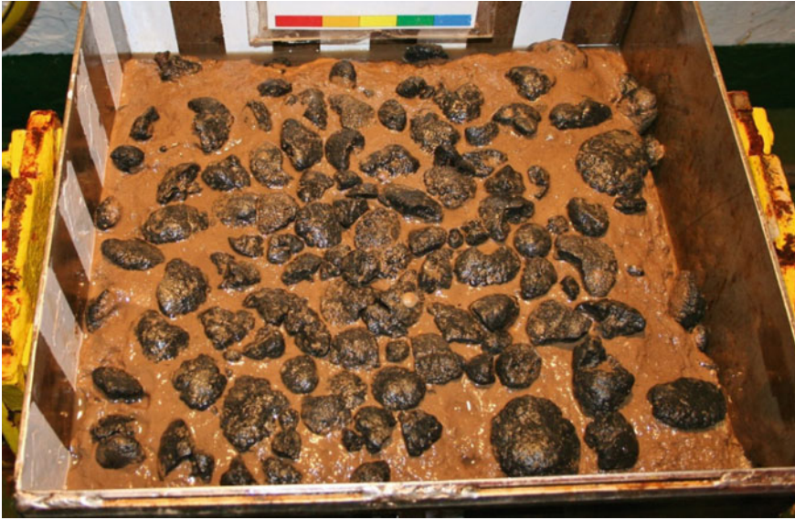
Fig. 45.2 Nodules deposited in oceanic sediment, extracted on a board of research vessel using a box corer
