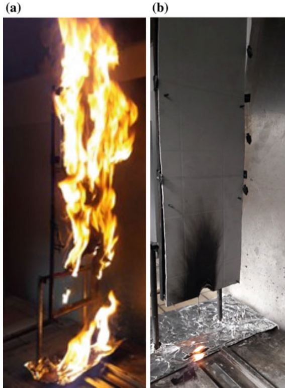
Fig. 49.4 Samples during the test: a PU1, b PC/ABS
