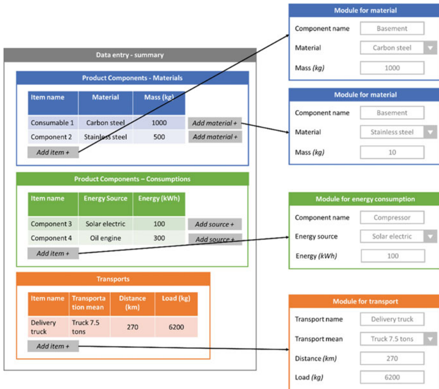
Fig. 14.5 Three kinds modules for Data Entry: a Module for material composition used for entering a new component (Consumable 1) and the same used for refining the Consumable 1 with a secondary material (i.e., stainless steel in addition to the more massive carbon steel), b module for energy consumption and c module for transport
