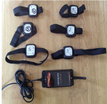
Fig. 39.1 ProMove mini sensors and Inertia Gate hub applied in the experiment
