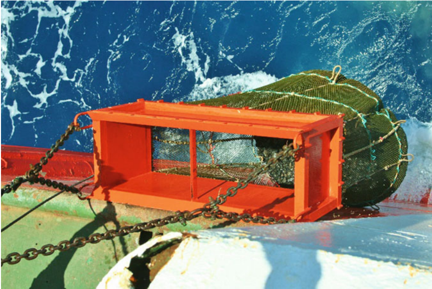
Fig. 45.3 Extracting larger amounts of nodules using a dredge
