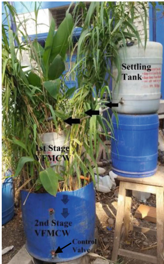
Fig. 3.2 Photographic view of experimental setup (VFMCW)
