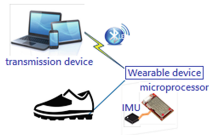
Fig. 4. A gait signal recording system
