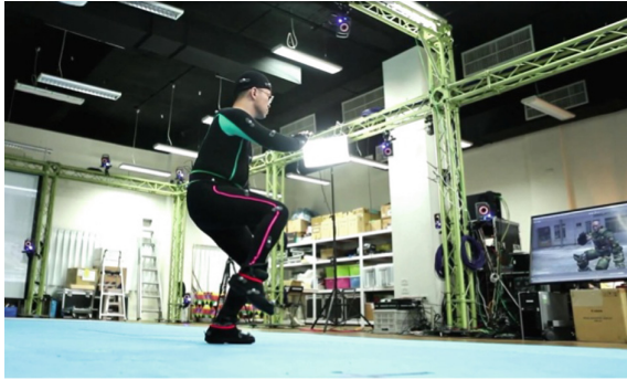
Fig. 1. Using Vicon cameras to record coach movement
