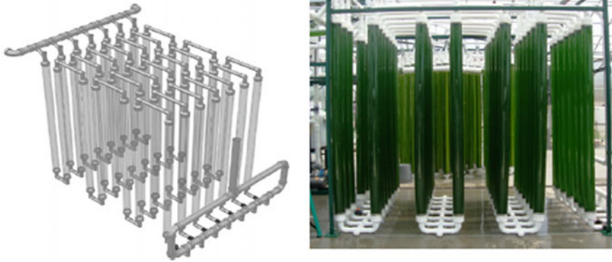
Fig. 14.5 Design template and image and image of vertical photobioreactors placed in series at 18 m 3 scale
