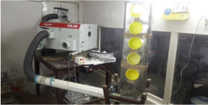
Fig. 8.1 Desiccant dehumidifier system
