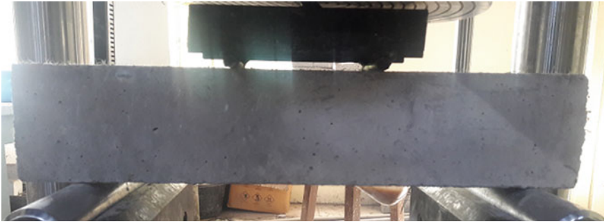
Fig. 2 Typical view of four-point bending test setup
