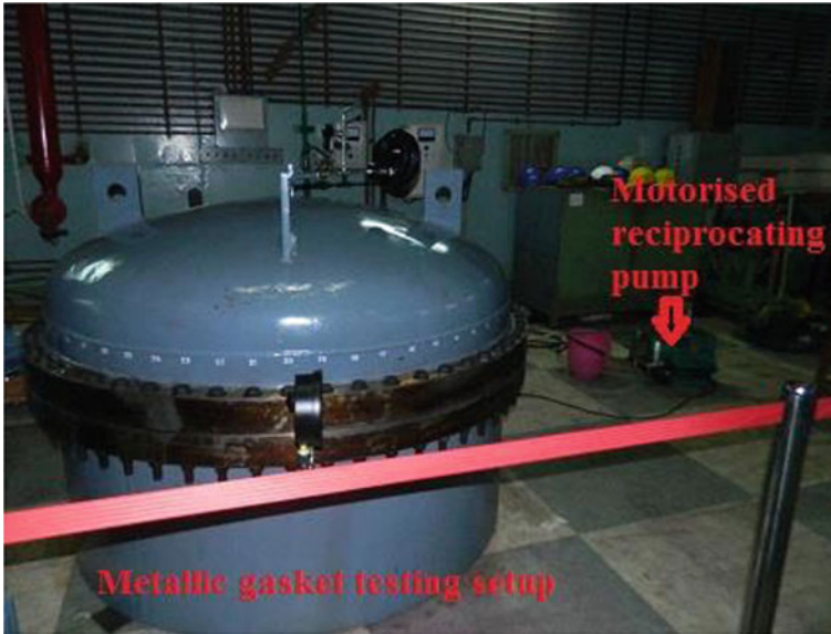
Fig. 8 Hydrotest set-up for metallic gasket
