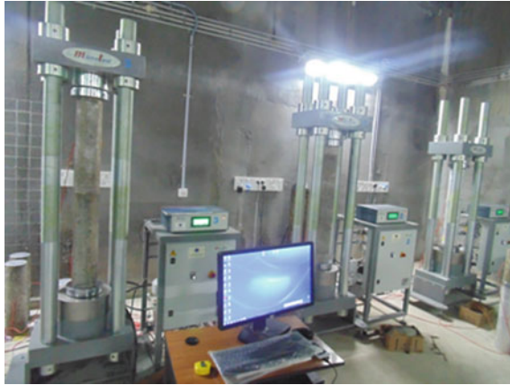
Fig. 1 Creep testing of concrete at CSIR-SERC
