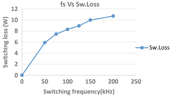
Fig. 10 Switching frequency versus switching loss
