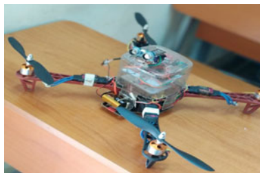
Fig. 18 Quadcopter with radar mounted
