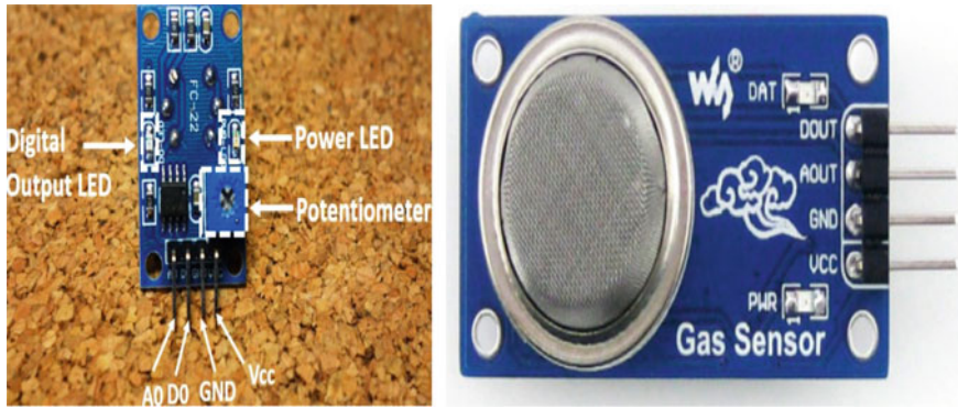
Fig. 4 MQ-2 gas sensor [6] (left side) and MQ-135 gas sensor [7] (right side)
