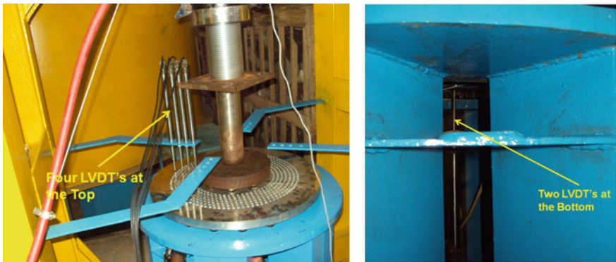
Fig. 6 Six LVDTs in the radial direction, four on top and two on the bottom surface of the test specimen
