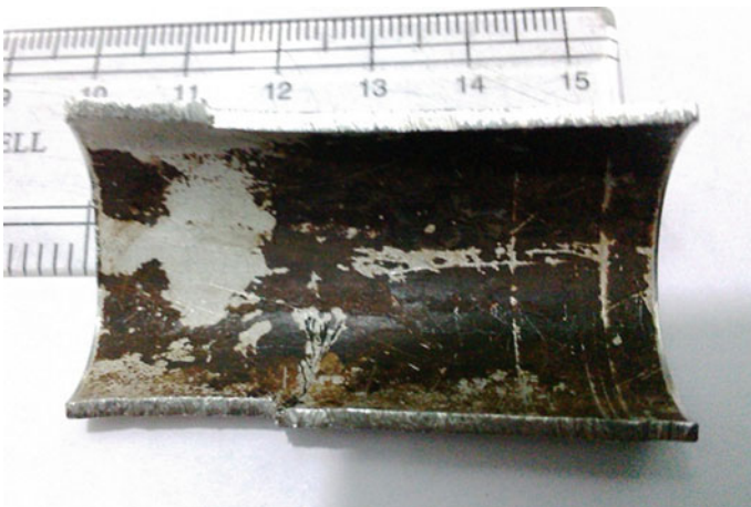
Photograph 4 Black adherent coating on the inside surface of the tube along with a bunch of cracks
