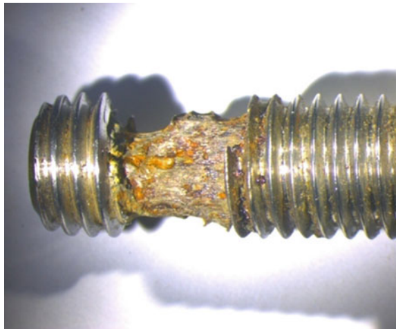
Photograph 7 a Bolt Sample given for detailed analysis. b Corroded Fastener still remaining in the filter
