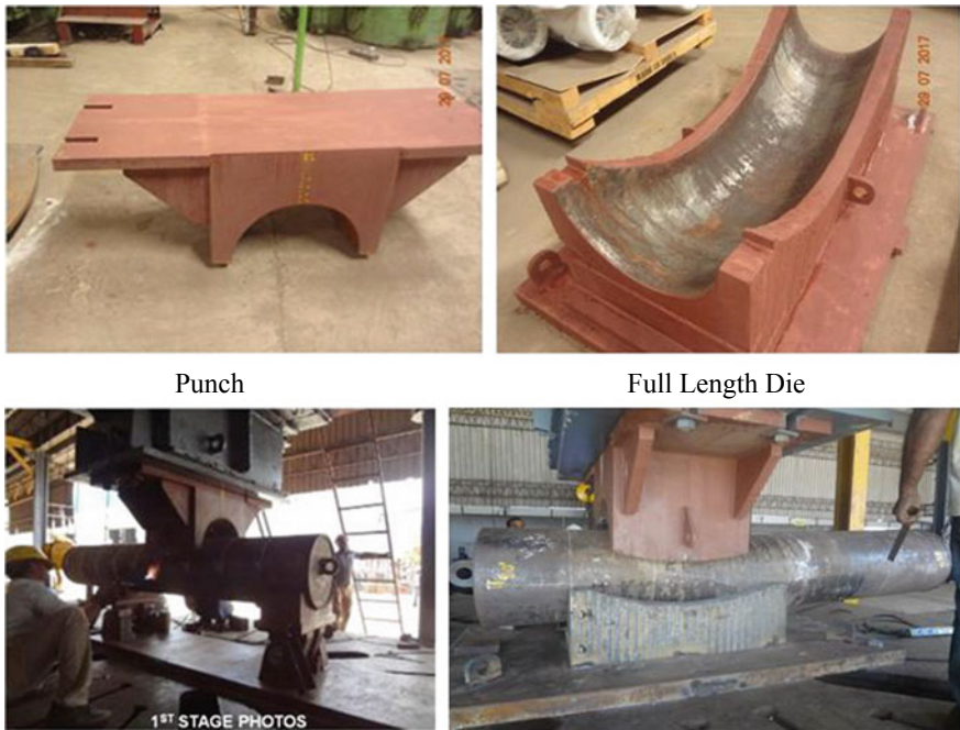
Fig. 4 Pressing of hot carbon steel pipe with end support die and full length die
