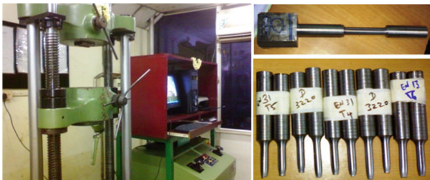
Fig. 5 Experimental setup of UTM & tested specimen
