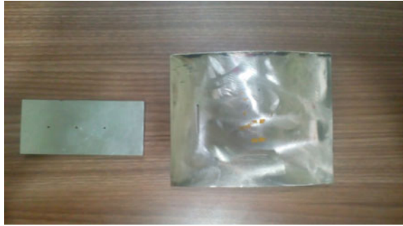
Fig. 12 Reference blocks for UT
