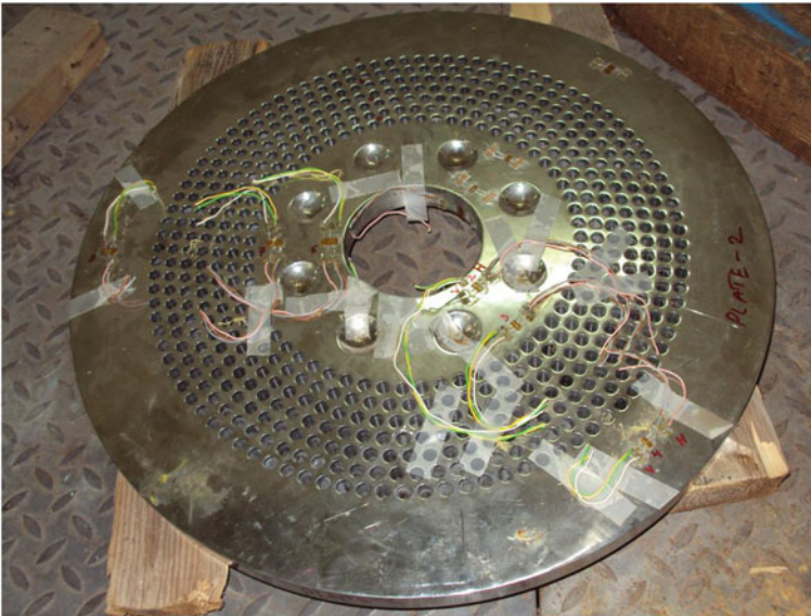
Fig. 8 Bidirectional strain gauges pasted on specimen No. 2
