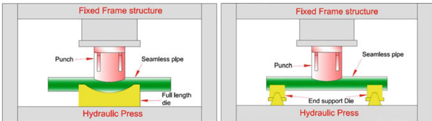
Fig. 5 Schematic arrangement of die and punch for hot forming
