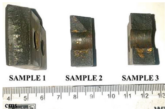
Fig. 2 Nomenclature and as-received fractured surfaces of blade root sections for failure analysis
