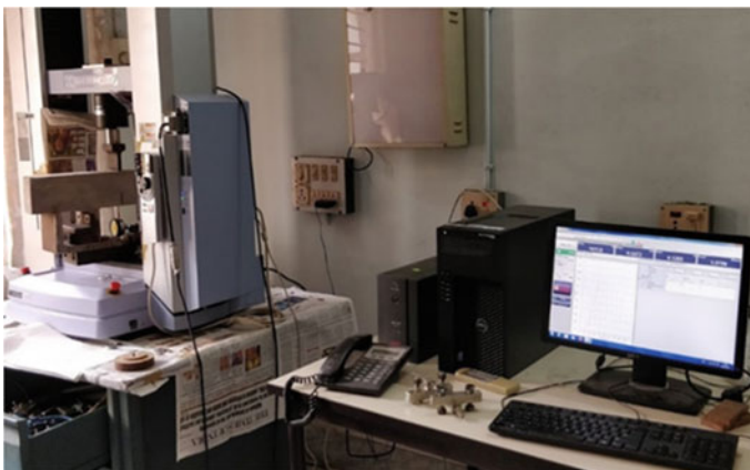
Fig. 5 Testing of specimens on a displacement control machine
