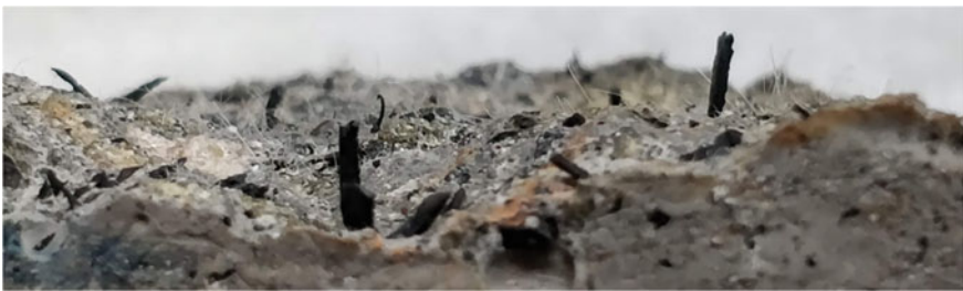
Fig. 10 Fractured surface of polypropylene fibre-reinforced rubcrete beams
