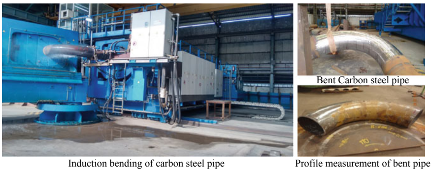
Fig. 6 Induction bending machine, bent carbon steel pipe, and profile measurement
