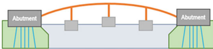
Fig. 15 Principle of bridge to adapt tidal variations
