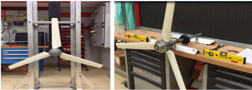
Fig. 20 Testing of balanced blade with rotor assembly
