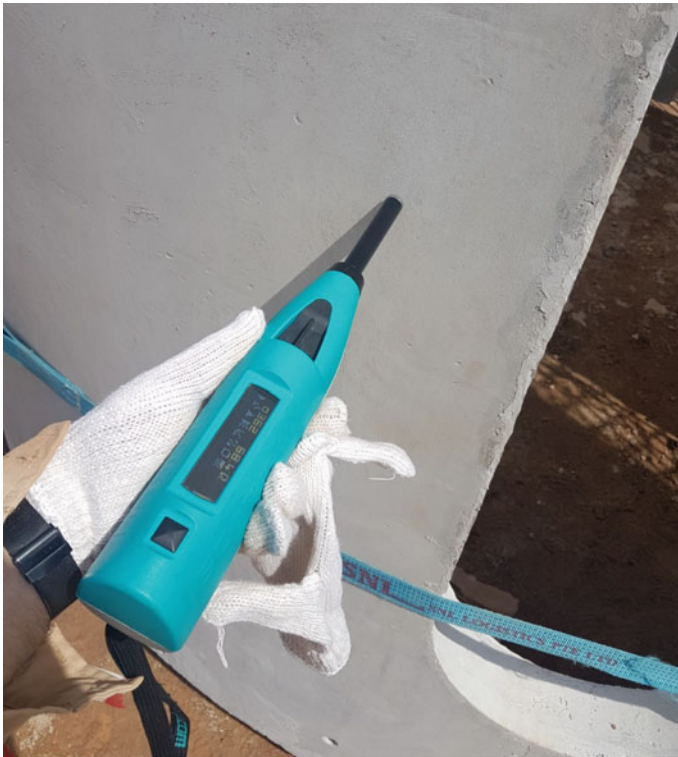
Fig. 4 Testing of in situ concrete strength using Schmidt rebound hammer
