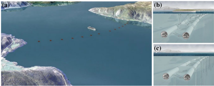
Fig. 4 Submerged floating twin tube tunnel: a aerial view of pontoon based support; b pontoon support; c tension-leg support. Courtesy NPRA
