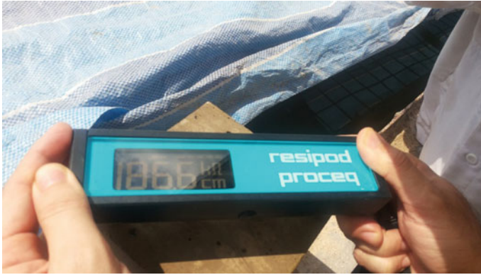
Fig. 3 Wenner Probe reading to measure concrete mix durability
