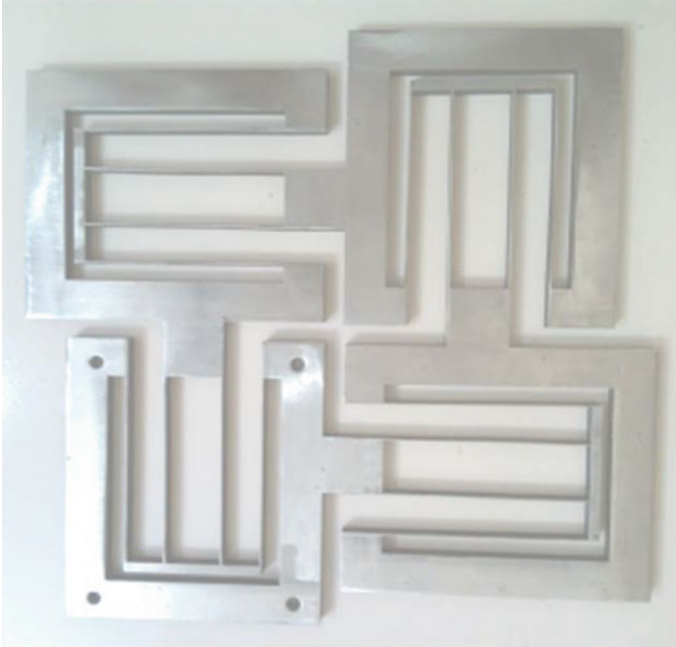
Fig. 13 Developed XY flexural mechanism
