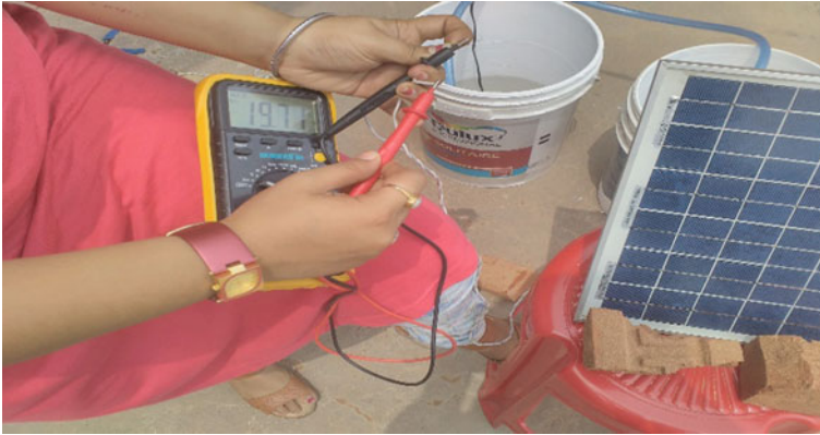
Fig. 4 Measurement of voltage obtained from solar cell
