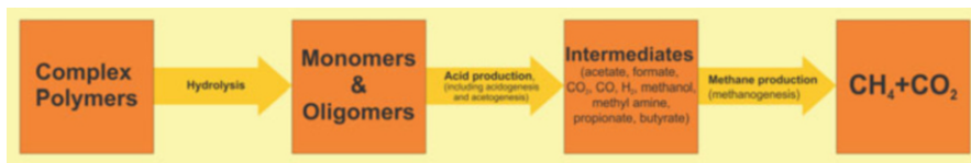
Fig. 4.1 Degradation process taking place during AD, i.e., hydrolysis, acidogenesis, acetogenesis, and methanogenesis. (Source: Merlin Christy et al. 2014; Chasnyk et al. 2015; Abdeslahian et al. 2016)
