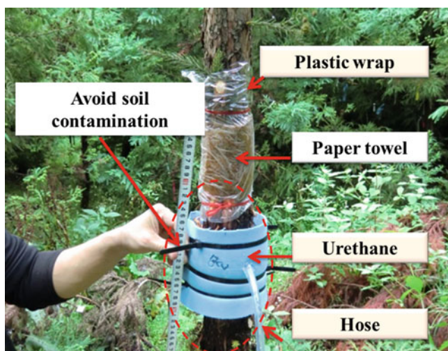
Fig. 4.5 A photograph of the ^{133}\text{Cs} application experiment on a representative 10-year-old cedar. A paper towel with 40 mL 0.01 M ^{133}\text{CsCl} solution was wrapped around bark at 1.2 m. A urethane sheet and hose were used to direct the stemflow to guttering
