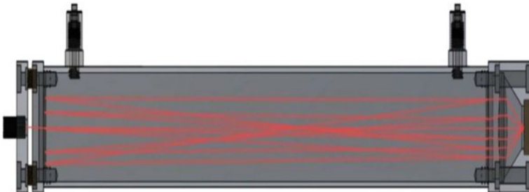
Fig. 4 Optical reflection diagram of the optical cavity
