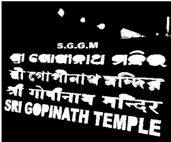
Fig. 4. Text components depicted as white and remaining parts of the image as black. An admissible amount of false positives is present in the final output.
