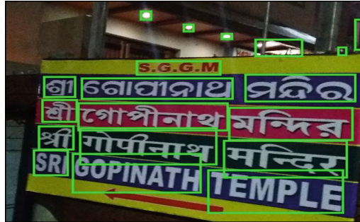
Fig. 5. Bounded words in the sample input image are considered as true positives. Some false positives are also bounded. No false negative occurs in this case.
