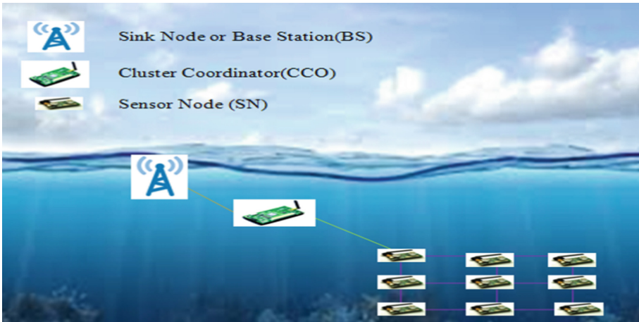
Fig. 1. Architecture of Multi hop Grid based Underwater Wireless Sensor Network
