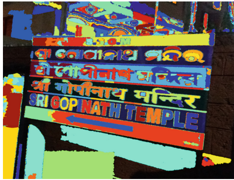
Fig. 2. The MSERs detected on the basis of local histogram analysis and dynamic region area selection.
