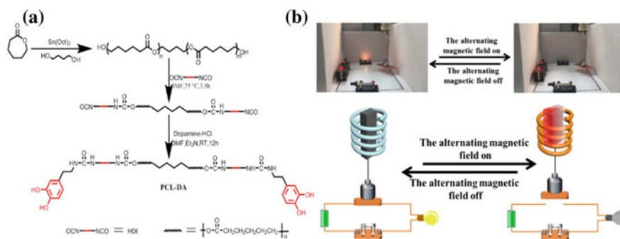
Fig. 21 a The preparation route of catechol-telechelic PCL and b the model of magnetic-triggered two-way shape-memory actuator used to realize on/off control in a circuit. Reprinted from [83] with permission from American Chemical Society
