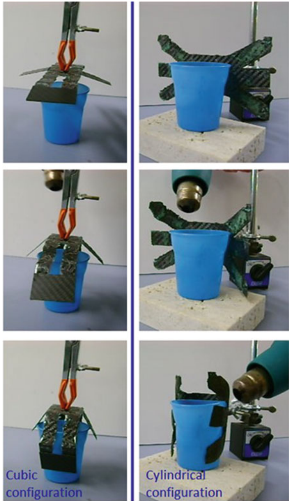
Fig. 9 Details of the shape-memory tests of the composite hands in cylindrical and cubic configuration [21]. Copyright 2016. Reproduced with permission from ASME
