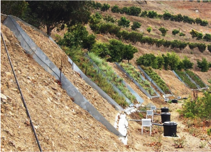
Fig. 7.3 Closed erosion and runoff plots used for the experiment
