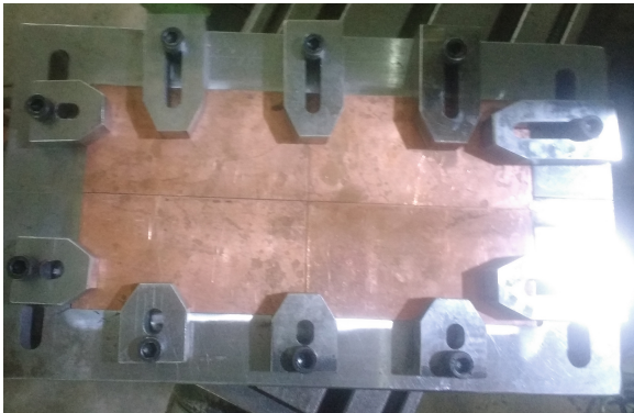
Fig. 7. FSW fixture with clamping
