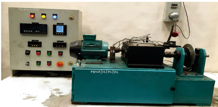
Fig. 2. Gear box test rig setup
