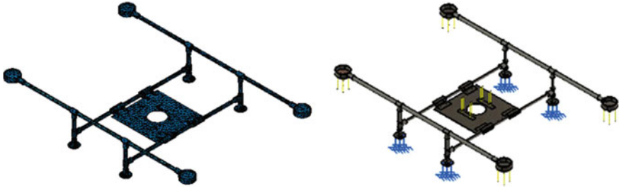
Fig. 24.2 Finite element model with boundary conditions
