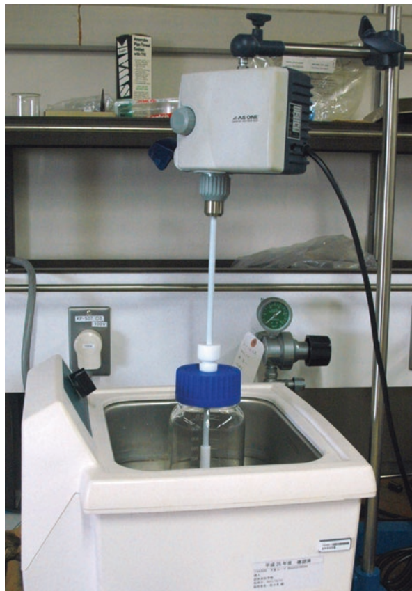
Fig. 7.5 A combination of mechanical stirrer and ultrasonic cleaner
