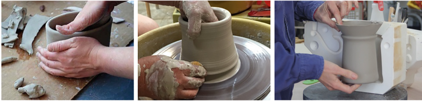
Fig. 1. Conventional ceramic production including hand-building, wheel-throwing, and slip-casting method in sequence. (Source: Shepherds Grove Studio)
