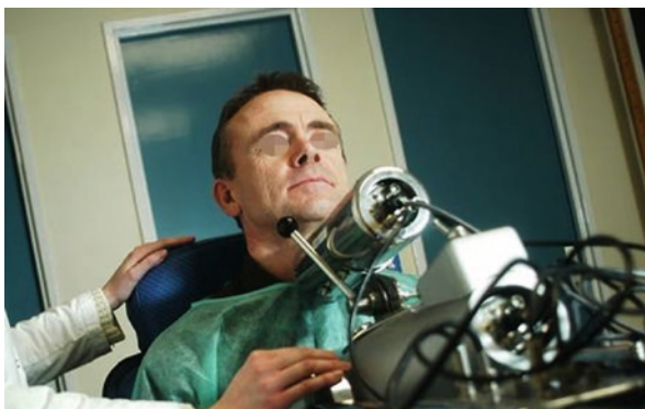
Fig. 15.3 In vivo measurement of 131 I activity in the thyroid at IRSN (© IRSN)
