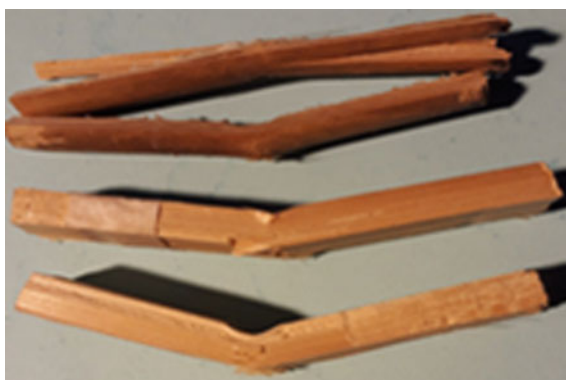
Fig. 5 Shows the nature of failure in culm after flexural test of the two species
