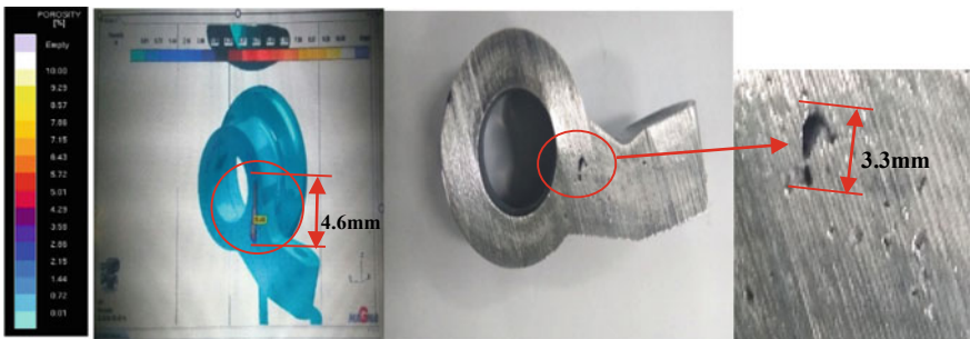
Fig. 6 Location 2, comparison between model and actual cross cut die casted power steering column products
