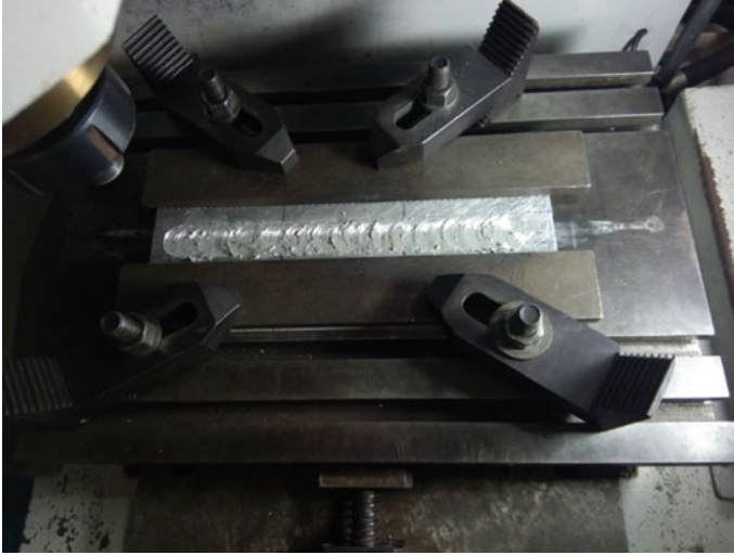
Fig. 2 Job setup with compacted 17-4 PH reinforcements
