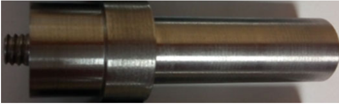
Fig. 1 H13 tool steel FSP threaded cylindrical pin tool
