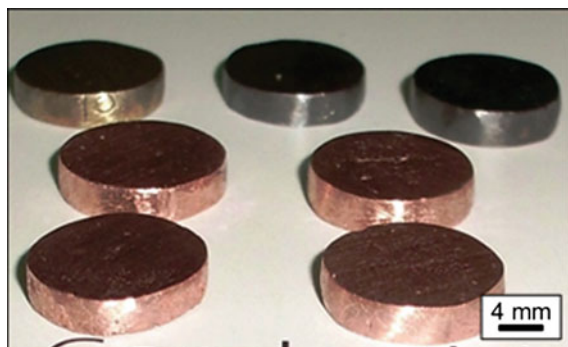
Fig. 2 Test samples for thermal conductivity measurement
