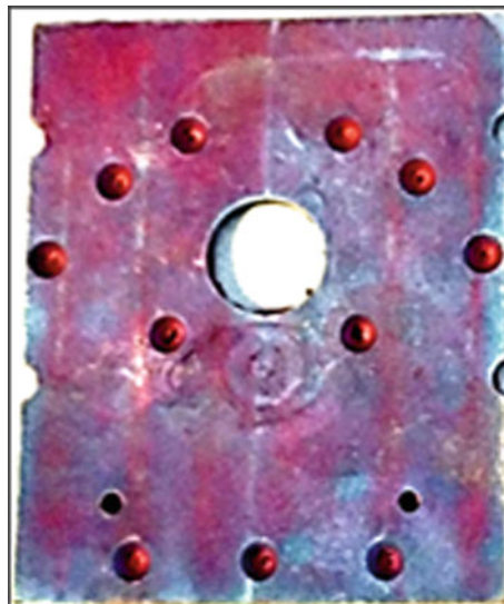
Fig. 8 Physical appearance of Cu-CNT samples after reliability testing for 500 thermal cycles
