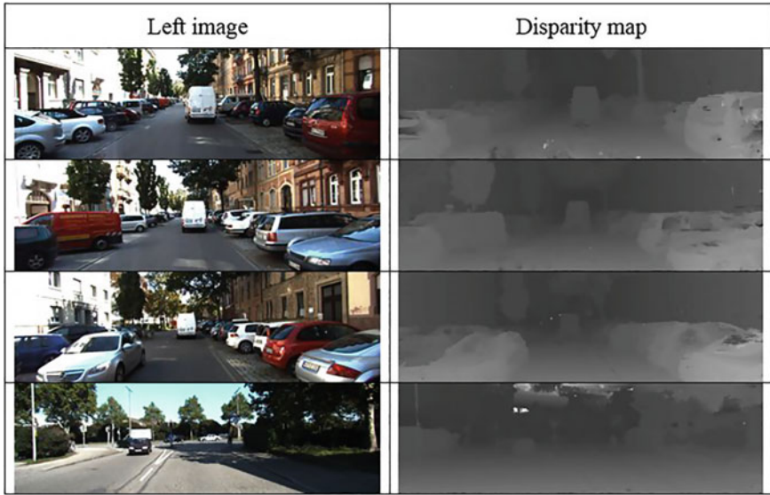
Fig. 4 The sample results of the KITTI training dataset from image number #000004_10-#000007_10 using the proposed algorithm
