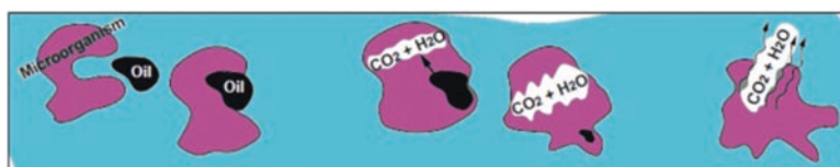
Fig. 5 Biodegradation of hydrocarbons (a) Microorganism eats oil or other organic contaminant. (b) Microorganism digests oil and converts it into CO 2 and H 2 O. (c) Microorganism gives off carbon dioxide and water into the environment
