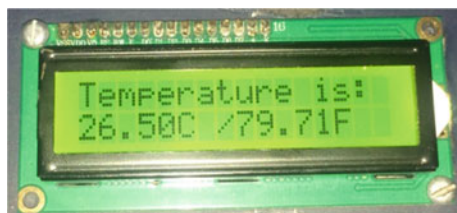
Fig. 7 Temperature displaying on LCD
