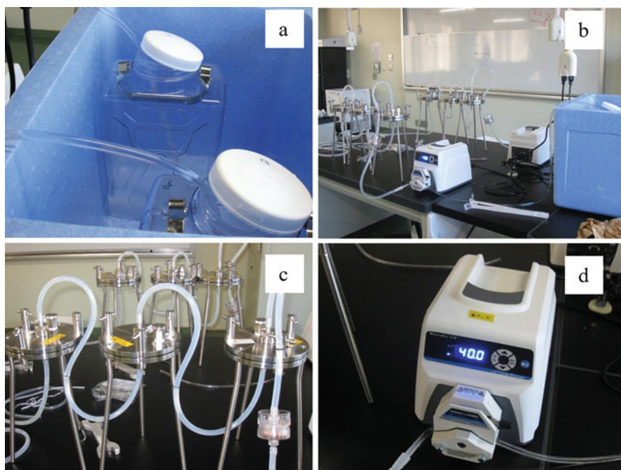
Fig. 1.5 Filtration of water. (a) Suction of water from tank, (b) and (c) sequential filtration using filtration system, and (d) peristaltic pump in use
