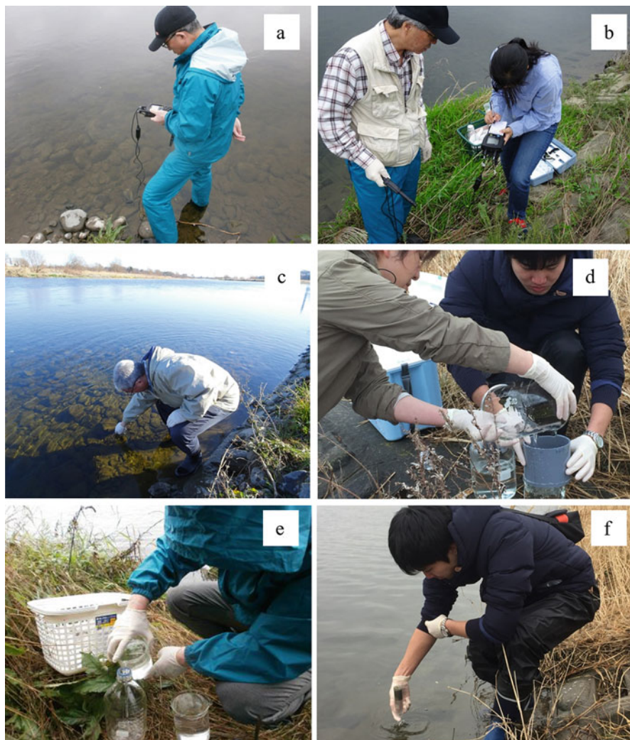
Fig. 1.1 Metagenomic sampling from a shallow river. (a) Monitoring environmental parameters, (b) recording environmental data, (c) sampling from surface layer of the river, (d) prefiltration using 100 \mu\text{m} filter, (e) pouring water sample into a sterile bottle, and (f) collection of sediments from riverbed of the Tama River, Tokyo, Japan
