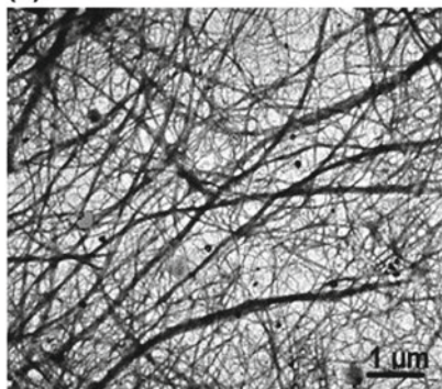
Fig. 2 Transmission electron micrographs from a dilute suspension of a cellulose nanofibrils from Opuntia ficus-indica [59], b cellulose nanocrystals from ramie fibers [26]
