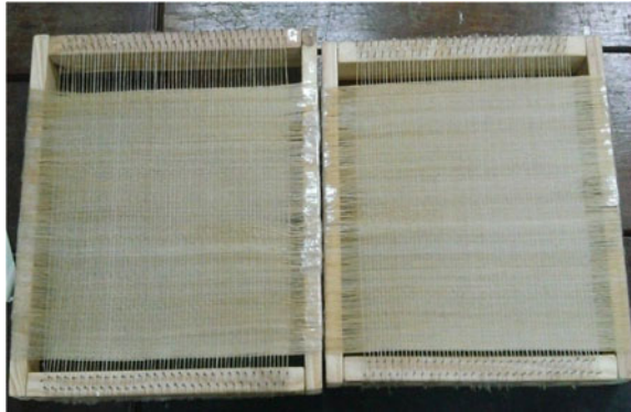
Fig. 7 Wooden block used for plain weave to produce natural fiber mat Thongpin et al. [77] Open Access
