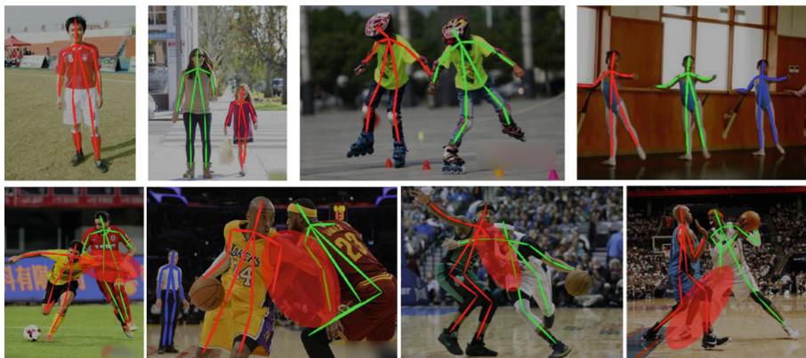
Fig. 1. Top: When the person in the scene are not overlapped, the recognition result is more accurate. Bottom: As shown in the red shaded area, if limbs are crossed, the skeletons are prone to disorder and loss. (Color figure online)
