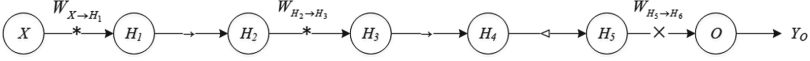
Fig. 11. The Capsule structure of a CNN, with “*” standing for convolution, “→” for identity transfer, “<” for tensor reshaping, and “×” for matrix multiplication.
