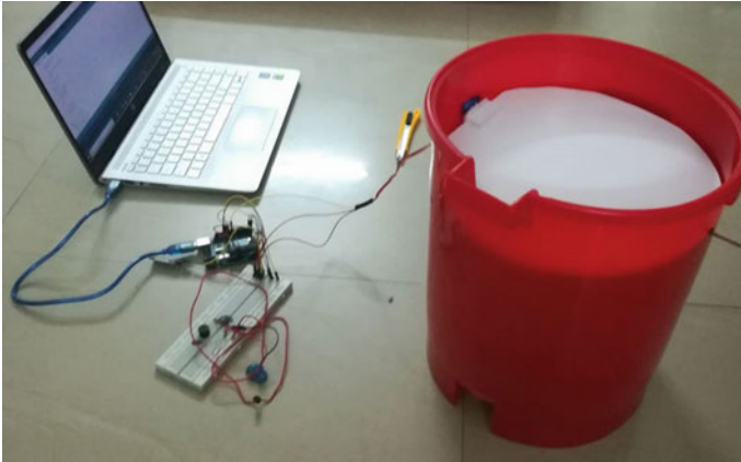
Fig. 9.2 RLC circuit with the bin used
