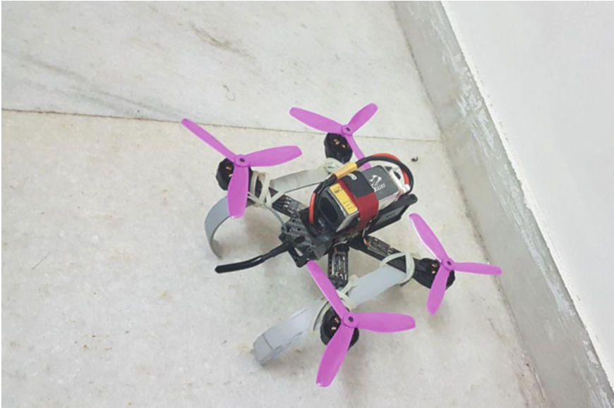
Fig. 15.14 Top view of the assembled quadcopter
