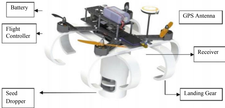
Fig. 15.1 CAD render of the developed drone
