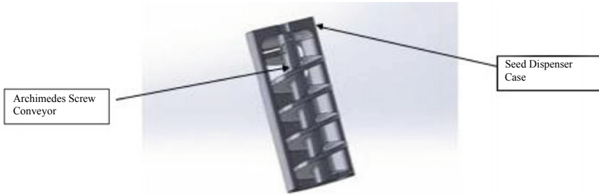
Fig. 15.2 Sectioned view of the seed dropper CAD model
