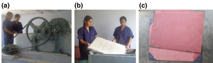
Fig. 18.5 a Slitting and soaking. b Paper base formation. c Paperboards
