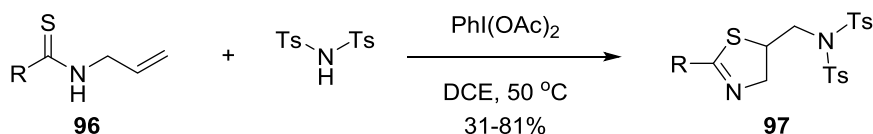
Scheme 6.24 Cyclization of N -allylthioamides with \text{Ts}_2\text{NH}
