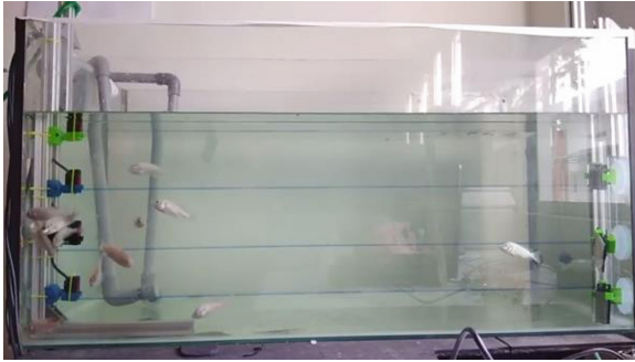
Fig. 1. Experiment setup using four photoelectric sensors in a fish tank.
