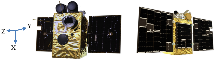
Fig. 1. The configuration of the satellite and the GNSS antennas installed on +z (left) and -z (right) side
