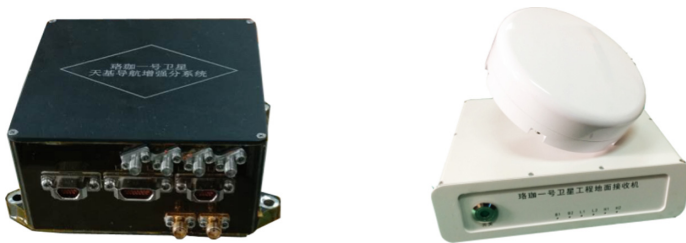
Fig. 2. The LEO navigation augmentation payload (left) and ground receivers (right) for Luojia-1A satellite
