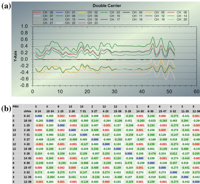
Fig. 4. a. The carrier phase double difference curves with stationary and moving dual-antenna b. The consistency detection statistics with stationary and moving dual-antenna
