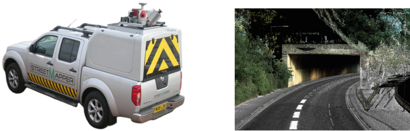
Fig. 3. StreetMapper and the color point cloud acquired
