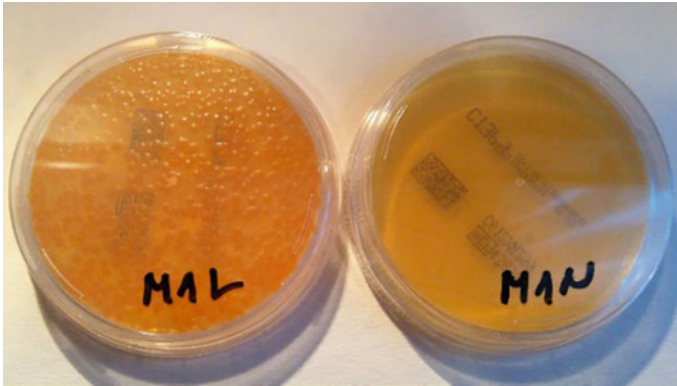
Fig. 3 Display of CT3P agar plate on the face and back sides of tested sample Fabric III
