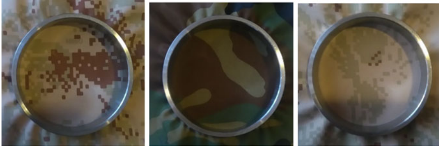
Fig. 2 Presentation of prepared samples for microbial barrier permeability testing
