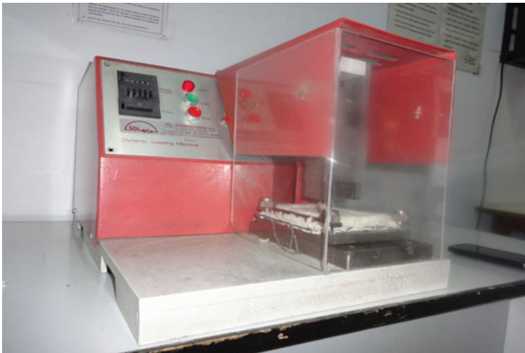
Fig. 7 Dynamic loading machine
