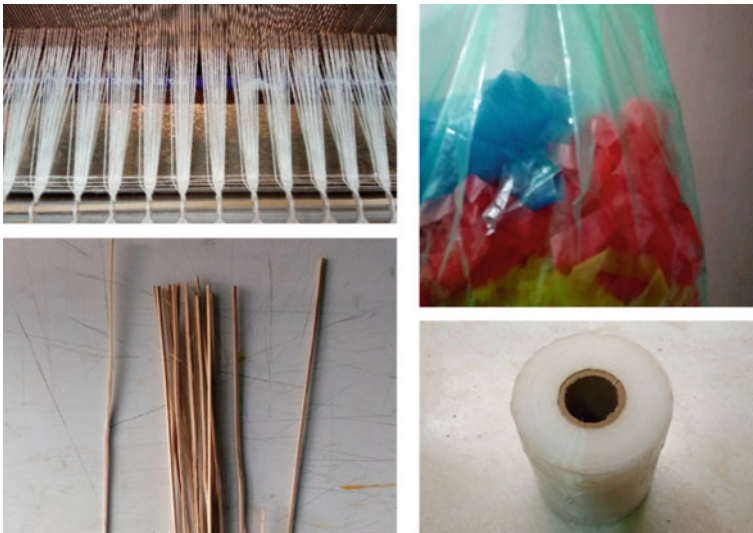
Fig. 13 Materials used: cotton for warp; polythene bags, shrinkable films, and bamboo sticks for weft (Courtesy: Shubhra Singh, 2016, NID, Ahmedabad)
