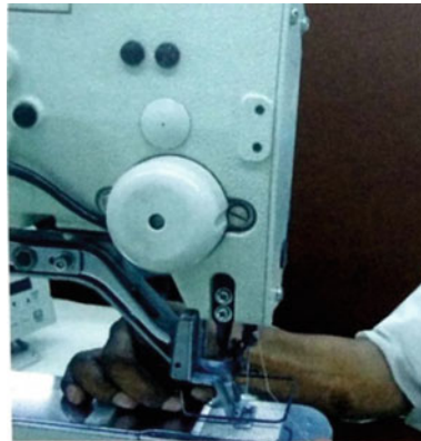
Fig. 3 Threading of bar-tacking machine
