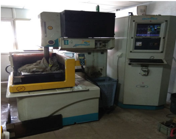
Fig. 32.1 Wire electric discharge machine [WEDM]
