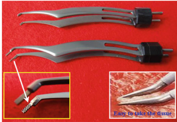
Fig. 29.7 Medical bipolars made of BMGs in the tip portion with a complex pattern [35]
