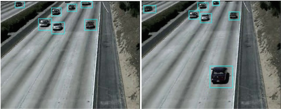
Fig. 3. Result of our model. We randomly extract three images from the video sequence, which are 2334 frame, and 2447 frame. From the results, we can see that the location where the foreground vehicles are connected has a good segmentation effect, and the position detection contour of each vehicle is reduced, indicating that the tracking result is more accurate.
