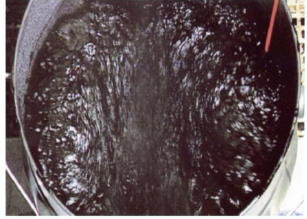
Fig. 2. Expansion of foamed asphalt
