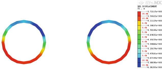
Fig. 4. The lateral displacement under design earthquake effect
