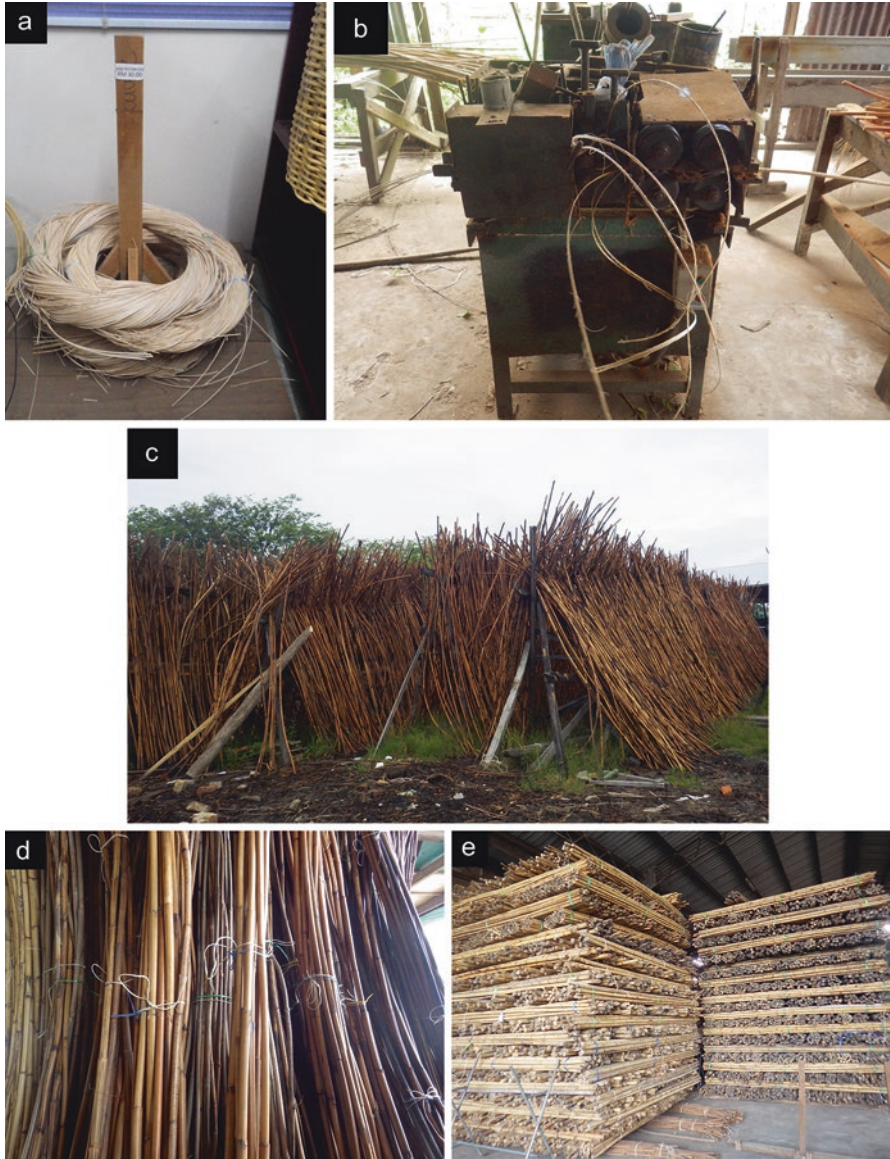
Fig. 22.7 Machine processing of rattans at the factory including: (a) bundles of rattan selling for RM30 per kg, (b) special machinery that peels and splits the rattan into several cores, (c) processed rattan drying, (d) bundles of rattan with different coloured string indicating the grade of the rattan, and (e) thousands of bundles of rattan being prepared for export to Singapore. (Photographs: Yayoi Takeuchi 2014)
