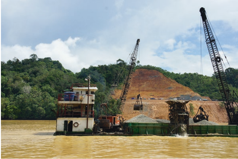
Fig. 2.7 Dredger for collection of sand from a river bed. (Photograph: Kuniyasu Mokudai 2013)
