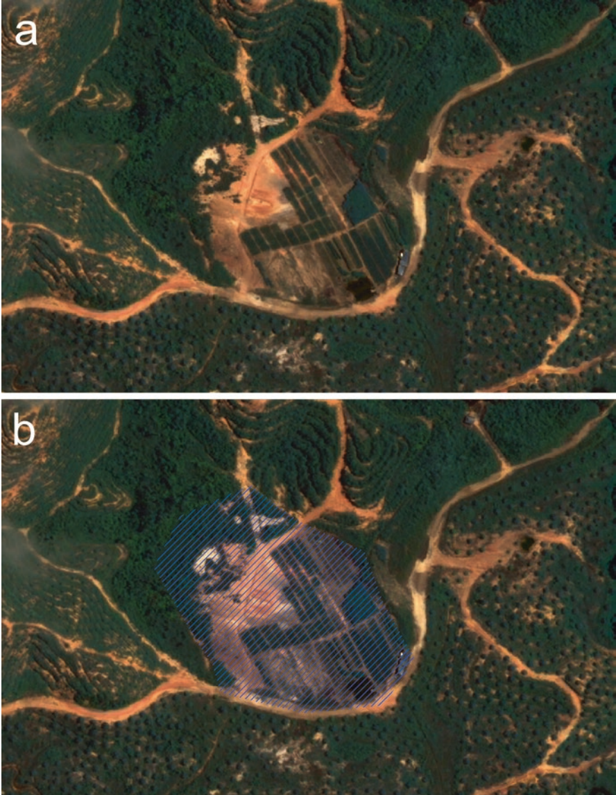
Fig. 3.9 (a) Satellite image used and (b) example of the resulting raster data set created in ArcGIS for the land-use subcategory of oil palm nursery
