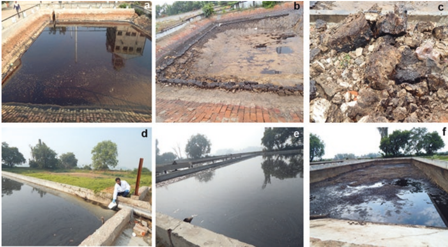
Fig. 17.1 Distillery waste (a) spent wash discharged after alcohol production; (b) solid material settle down in the bottom of storage tank as spent wash sludge; (c) large view of the spent wash sludge (d-e) anaerobically digested spent wash in collection tank (f) digested sludge discharged after biomethanation of spent wash
