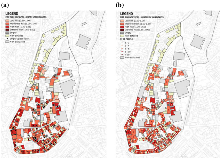
Fig. 10 Second level analysis: FR_I results with empty upper floors (a) and number of building occupants (b)
