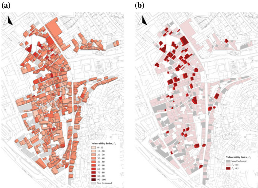
Fig. 2 Vulnerability index distribution (a) and identification of the building façade walls with vulnerability index values equal or higher than 45 (b), adapted from Aguado et al. (2018)
