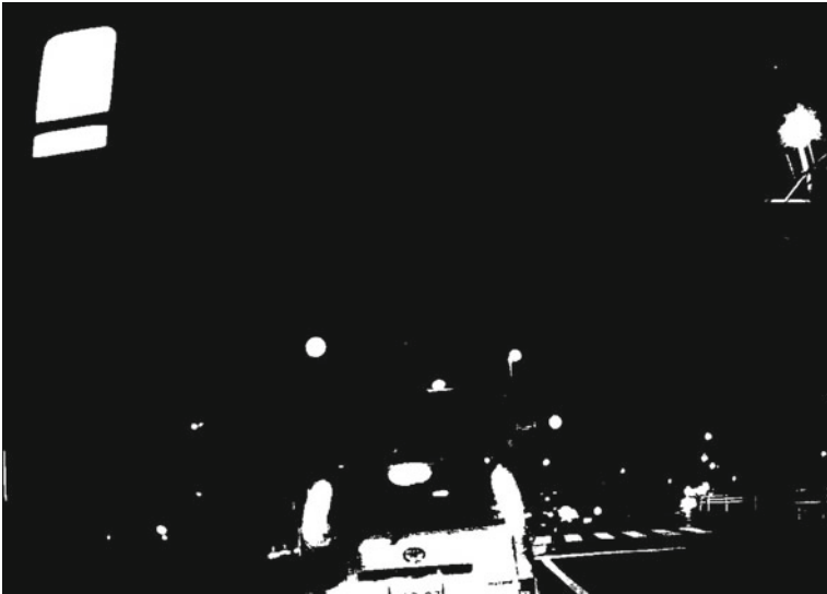
Fig. 7 Binary image showing spots of high brightness
