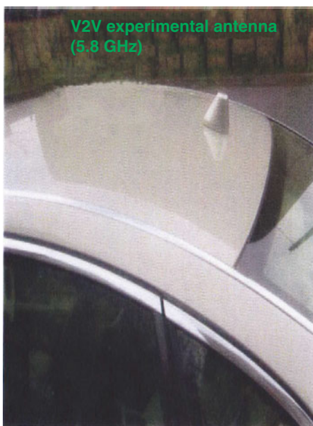
Fig. 2 Experiment using vehicle-to-vehicle communication by DSRC to avoid crashes at a crossing
