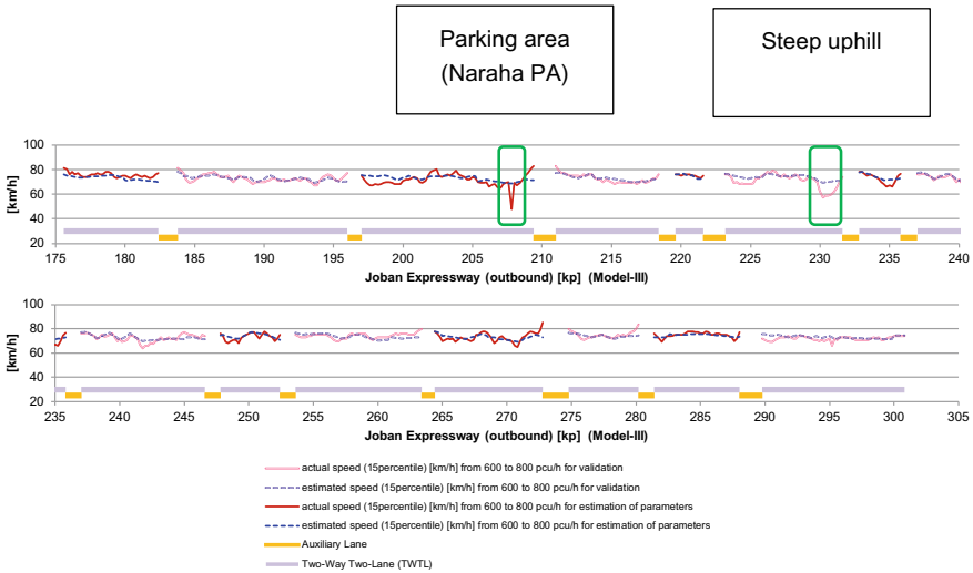
Fig. 4 Cross-validation of speed profiles based on Model III with estimated parameters for flow rates from 600 to 800 pcu/h on the Joban Expressway
