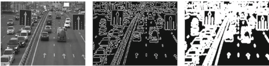
Fig. 2 Image enhancement of busy road (here density in right lane is given 47%)
