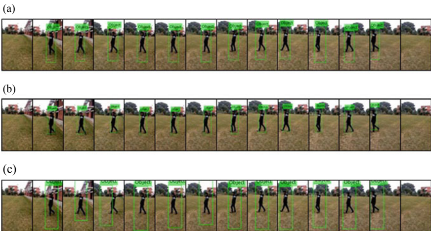
Fig. 2 Sequence of frames with blob using a HAAR, b LBP, and c HOG
