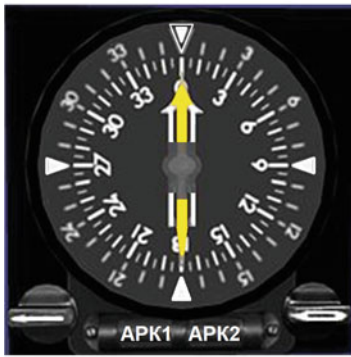
Fig. 2.5 Indication on the RMI and flight pattern “to NDB”
