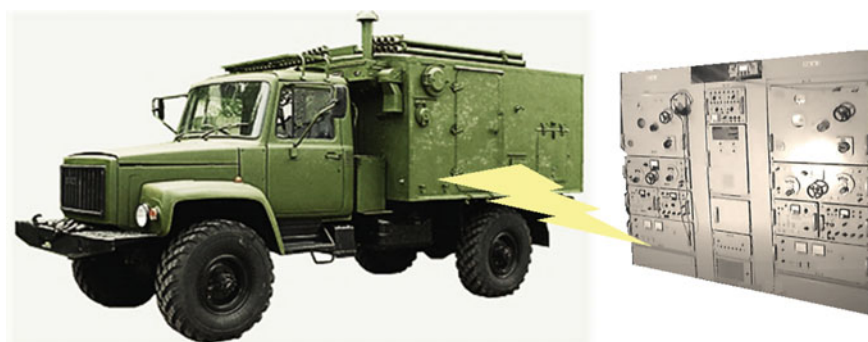
Fig. 2.16 Mobile variant of NDB placement
